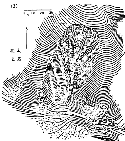
第33図 扇状堆積(地下水流運積)を示す崩壊 Fig. 33 The landslide in which has not deposits due to transportation of ground-water.(formed aluvial fan)
